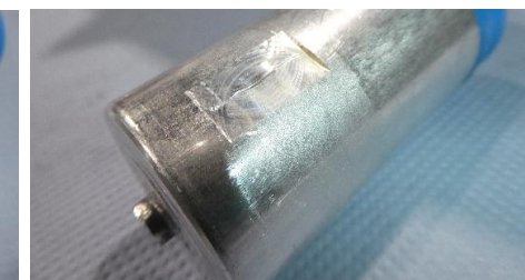
Cell cleaned after venting
