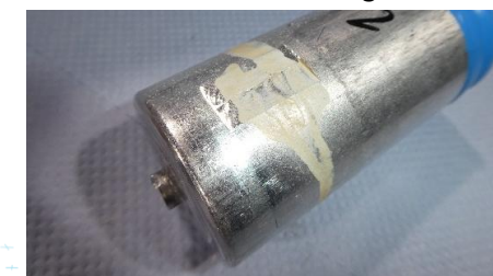
Cell vented during test
